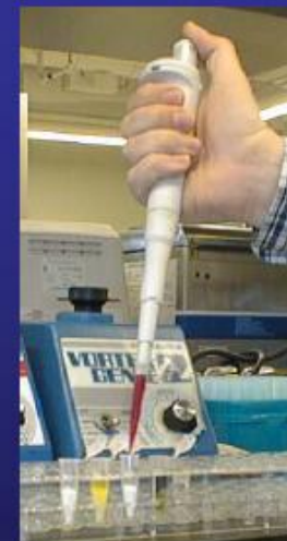
3) Mix a portion with a sorbent
