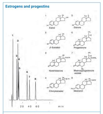
YMC-Pack  $C_8$  (Octyl) (5  $\mu m,\,12$  nm) 250 x 4.6 mm ID OC12S05-2546WT acetonitrile / THF / water (46/4/50) Column:
