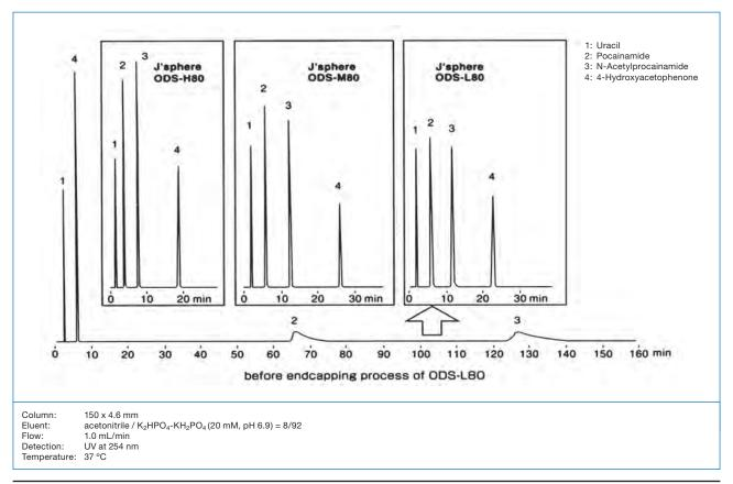
Three types of ODS are processed by endcapping technology to minimize the effect of residual silanol as much as possible.
