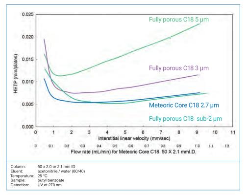
Meteoric Core C18 has high column efficiency which is almost equivalent to sub-2 µm columns over a wide range of flow rates.
