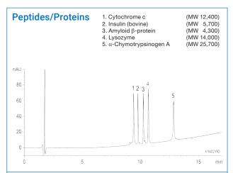
Column: Meteoric Core BIO (2.7  $\mu$ m, 16 nm) 150 x 2.1 mm ID
