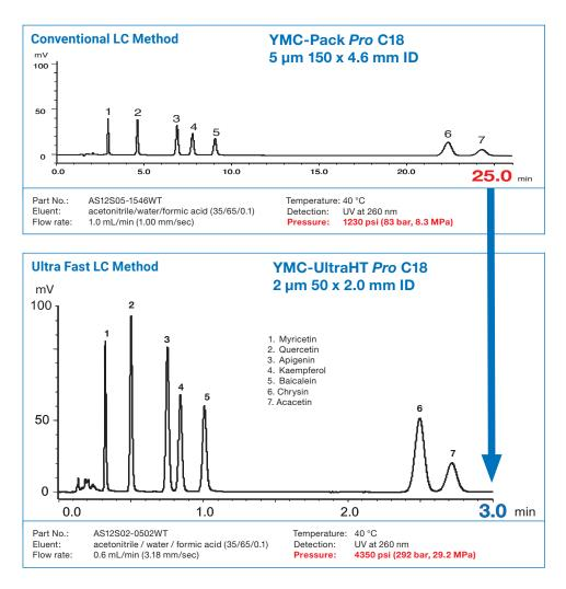
Due to the production processes used to manufacture YMC-Pack Pro-Family, methods can be easily downscaled with unchanged selectivity.
