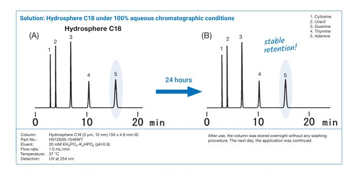
Its "hydrophilic" C18 surface gives Hydrosphere C18 the capability to show stable retention times even after 24 hours under these chromatographic conditions.
