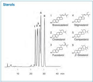
YMC-Pack ODS-AL (5 µm, 12 nm) 250 x 4.6 mm ID Column:
