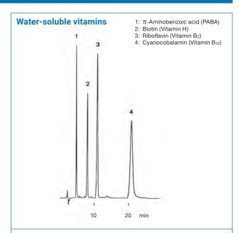
Column: YMC-Pack Ph (5  $\mu m,\,12$  nm) 150 x 4.6 mm ID PH12S05-1546WT
