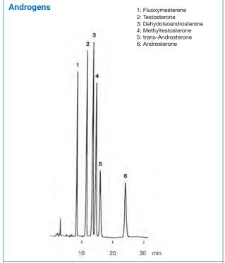
J'sphere ODS-L80 (8 nm, 4  $\mu$ m) 150 x 4.6 mm ID Column:
