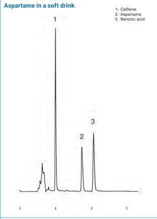
YMC-Pack CN (5  $\mu m,\,12$  nm) 250 x 4.6 mm ID CN12S05-2546WT
