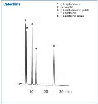
J'sphere ODS-M80 (8 nm, 4  $\mu$ m) 150 x 4.6 mm ID JM08S04-1546WT Column:
