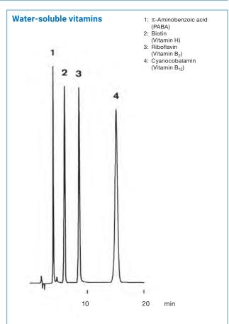
YMC-Pack TMS (5 μm, 12 nm) 150 x 4.6 mm ID
