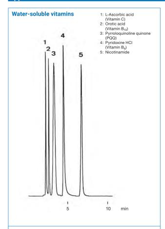
YMC-Pack TMS (5 µm, 12 nm) 150 x 4.6 mm ID
