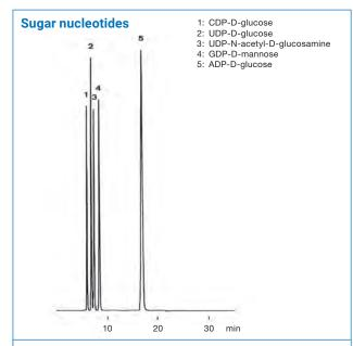
Column: Part No.: YMC-Pack Ph (5  $\mu$ m, 12 nm) 250 x 4.6 mm ID PH12S05-2546WT
