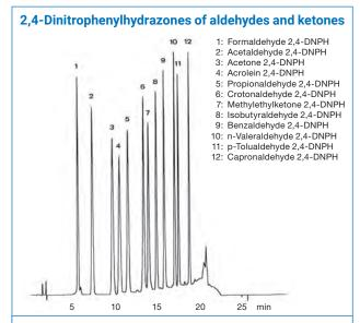
YMC-Pack C<sub>4</sub> (5 µm ,12 nm) 150 x 4.6 mm ID Column:
