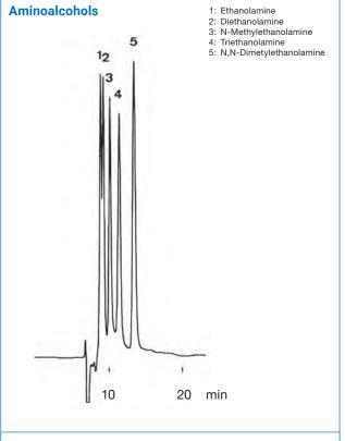
Column: YMC-Pack Polymer C18 250 x 6.0 mm ID Part No.: PC99S06-2506WT
