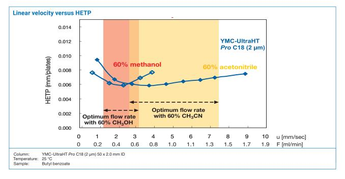
Since YMC-UltraHT columns provide substantially lower pressure drop than most competitive 2  $\mu$ m or sub-2  $\mu$ m media, high flow rates can be achieved without generating excessive back pressure and without the need for specialised equipment. Nevertheless, 3 mm ID columns are less
