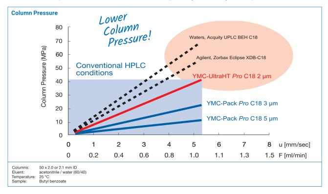
The introduction of YMC-UltraHT Pro C18 2 µm allows easy downscaling of existing methods which use YMC-Pack Pro C18 3 µm and 5 µm.
