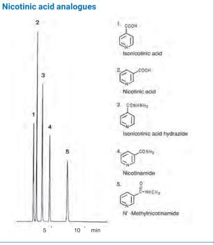
YMC-Pack C8 (Octyl) (5  $\mu m,~12~nm)$  150 x 4.6 mm ID OC12S05-1546WT acetonitrile / 20 mM KH2PO4 (5/95) Column:
