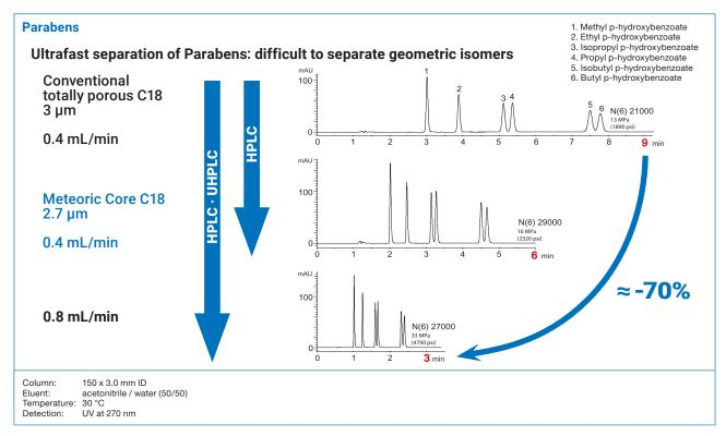
Meteoric Core C18 can shorten the analysis time by two thirds compared to a conventional totally porous C18 column with the same column dimensions and under the same analytical conditions. In addition, it maintains
