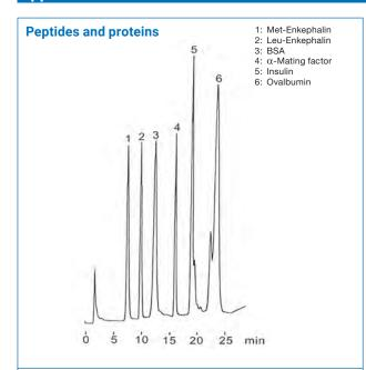
Column: Part No.: YMC-Pack Polymer C18 150 x 4.6 mm ID PC99S06-1546WT
