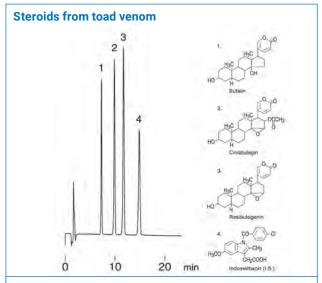
YMC-Pack ODS-AL (5 μm, 12 nm) 150 x 4.6 mm ID Column:
