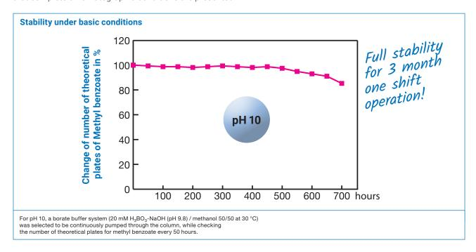
Basic eluents may significantly affect silicas and traditional bonding chemistries. Therefore, stability data should be considered only after verifying that the buffer system used maintains the selected pH during preparation and use. Furthermore, it must be verified that the eluent is not
