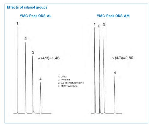
The separation factor  $(\alpha)$  of internal standards methylparaben / 2,6-dimethylpyridine for YMC-Pack ODS-AL, which is not endcapped is different to that of YMC-Pack ODS-AM. Due to the residual silanol groups, YMC-Pack ODS-AL shows higher retention of pyridines.
