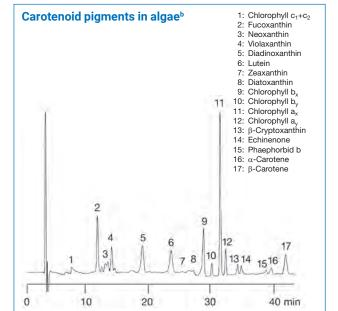
Column: YMC Carotenoid (5 µm) 250 x 4.6 mm ID
