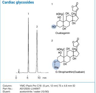
Flow: 1.0 mL/min Detection: UV at 220 nm, 0.26 AUFS 37  $^{\circ}\text{C}$ Temperature:  $5 \, \mu L \, (0.2, \, 0.4 \, mg/mL)$
