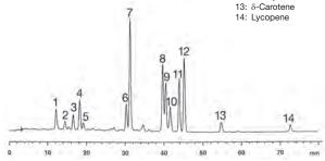
YMC Carotenoid (5  $\mu m)$  250 x 4.6 mm ID CT99S05-2546WT Column:
