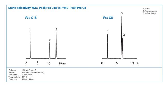
The reversed elution order of triphenylene and o-terphenyl for the shorter C8 chains of YMC-Pack *Pro* C8 illustrates the different steric recognition for steric-demanding substances.
