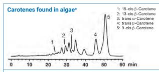
Column: YMC Carotenoid (5 µm) 250 x 4.6 mm ID
