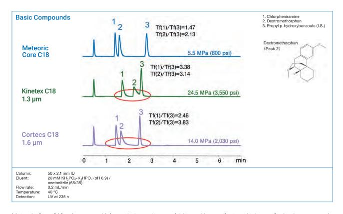
Meteoric Core C18 columns are high resolution columns which provide excellent peak shapes for basic compounds compared to competitors' sub-2 µm core-shell columns. Chromatographers can expect ultrafast analysis of basic compounds with highly quantitative and sensitive analysis when using Meteoric Core C18.
