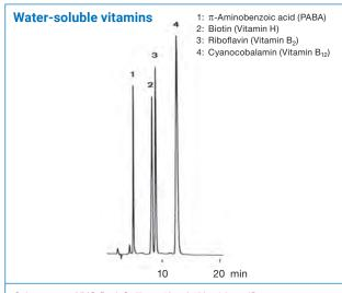
YMC-Pack C $_4$  (5  $\mu m,\,12$  nm) 150 x 4.6 mm ID BU12S05-1546WT Column:
