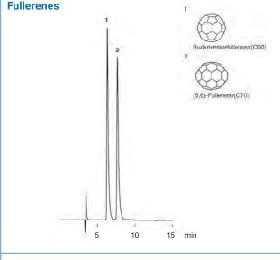
Column: YMC-Pack Ph (5 µm, 12 nm) 150 x 6.0 mm ID PH12S05-1506WT
