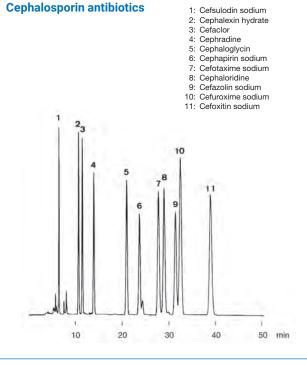
J'sphere ODS-M80 (8 nm, 4  $\mu$ m) 250 x 4.6 mm ID JM08S04-2546WT Column:
