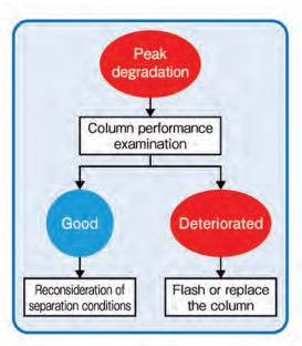
YMC provide sufficient analytical information, including sample concentration, in the Column Inspection Reports to allow customers to evaluate the performance of the column using standard compounds.
