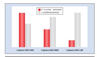
Hydrophobicity (indicated by k' for n-octyl benzene) and H-bonding capacity (indicated by a of caffeine/phenol) of J'sphere ODS columns.
