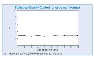
interactions with residual silanol groups. 2,6-dimethylpyridine, however, represents a lipophilic amine compound which has a high potential of unspecific interaction with unreacted acidic silanols. An increase in retention of 2,6-dimethylpyridine and hence lower α-values would indicate incomplete C18 bonding and/or ineffective endcapping. YMC specifies for ODS-AM that the statistical a-value of methylparaben and 2,6-dimethylpyridine be 2.77 +/- 0.20.
