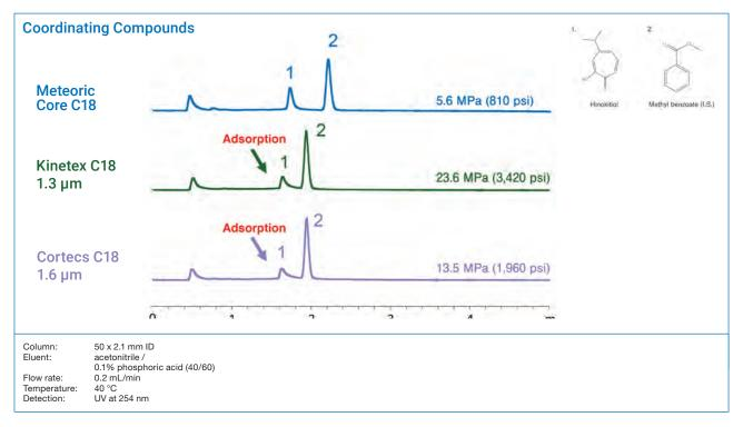
Meteoric Core C18 is able to provide excellent peak shapes for coordinating compounds which are often adsorbed by a column, as a result of a strong interaction with impurities such as trace amounts of metal ions. Meteoric Core is suitable for the quantitative analysis of coordinating compounds.
