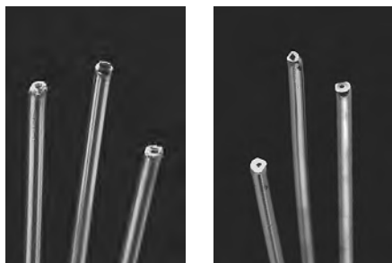
AVOID UNEVEN ENDS AND BURRS, DUE TO FILES (L) AND PLIER CUTS (R)
