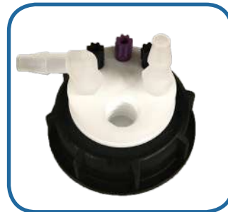
SW55-3-C-2L : 3 entries 1/8", a charcoal cartridge emplacement and 2 threaded barbed fittings
